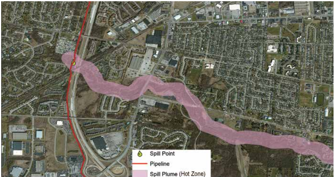
Based on the topography of the area, the product released from a liquid pipeline spill can travel a considerable distance from the point of the release.
